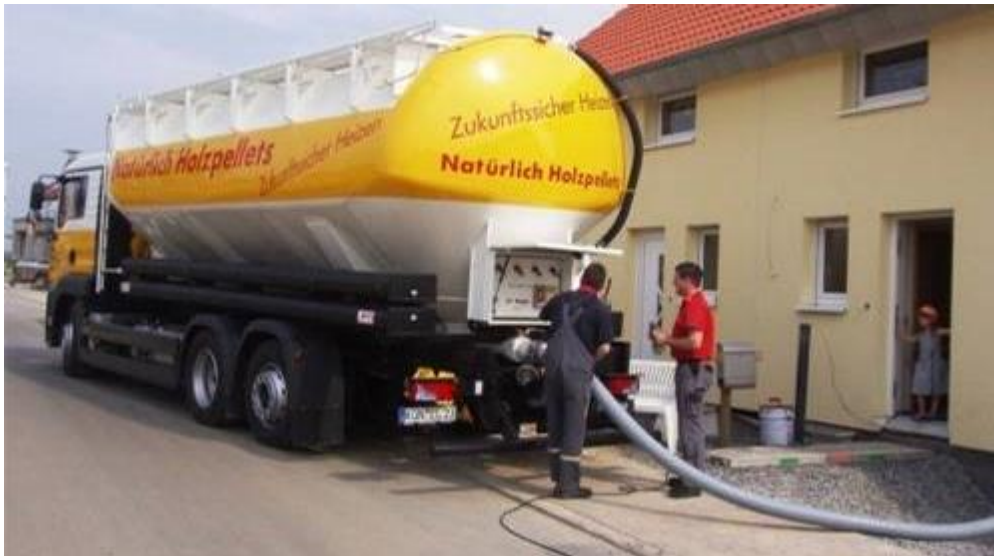
Picture 7: Special lorry for wood pellets. These are pumped through the grey hose by compressed air. Photo archive DLM
