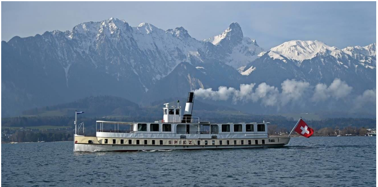
Fig. 3: Trial run of the re-steamed screw ship "SPIEZ". The ship was built in 1901 by the Swiss company Sulzer Ltd. as a coal-fired steamship. In 1952, it was converted to diesel operation. The old steam engine was scrapped. The new steam plant with automatic boiler and the new remote controlled steam engine allows the same staffing as on a motor vessel. Photo: Robert Horlacher
