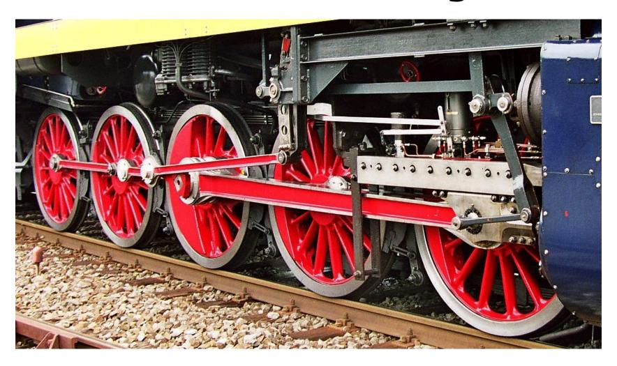
Replacing the old plain bearings with modern roller bearings improved adhesion, reduced maintenance and eliminated oil losses.
