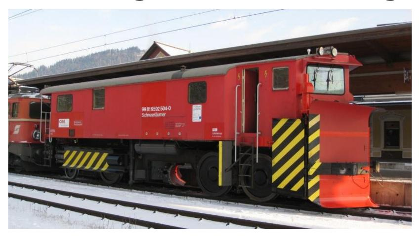
The snow ploughs are pushed by locomotives. The maximum speed allowed for snow ploughing is 60 km/h. However on test runs 100 km/h have been reached without any problems.
