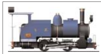
Fig. 28: New oil fired steam locomotive as proposed to the Indian Railways for the Darjeeling line. The distinct external appearance, which is characteristic for the Darjeeling Railway was intentionally retained in view of the UNESCO World Heritage status.
