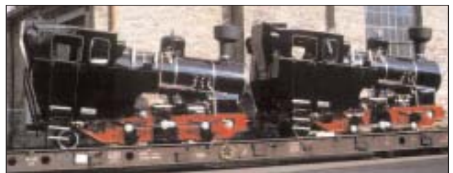
Fig. 15: Environment-friendly transport of environment-friendly products. Two brand new rack steam locomotives built in 1996 for the Schafberg Railway, ready to be sent by rail transport
